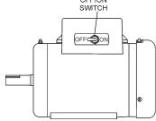
Figure 23. Electric Motor ON/OFF Switch (OFF Position)
